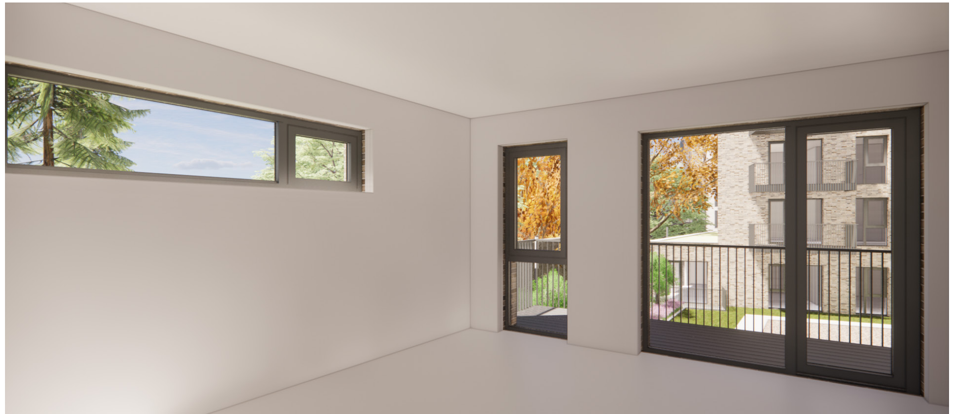
Figure 32 - Internal view from Block 04 looking south west showing clerestory window to prevent overlooking to the south.
